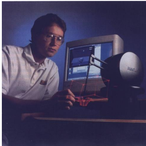
Geomagic® Phantom® Premium (ex Sensable Techn. 1993-2012) Now 3D Systems A similar device (Falcon) is available and used in our lab for rehabilitation
